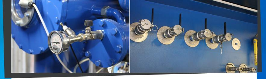
The combination of this techniques is what makes the reclaiming or regeneration treatment highly ef-ficient and reliable on the recovery of the Physical, Chemical and Electrical properties of the treated oil and the effective cleaning of the Transformer core and windings. With dehydration and vacuum degassing we can re-duce the ppm on or under the limits permitted, the dissolved or emulsified water in the oil, while we de-gasses and remove the most volatile acids in the oil.
